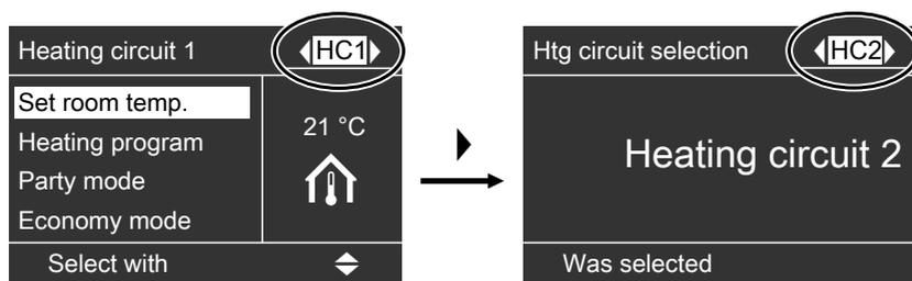
The heating circuits are marked at the factory as **"Heating circuit 1" (HC1)** and **"Heating circuit 2" (HC2)**.
