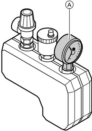
1. Check the heating system pressure at pressure gauge (A):
